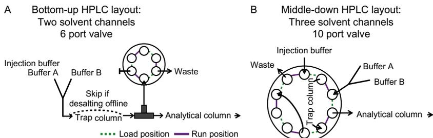
**Figure 5** Valve layouts for bottom-up and middle-down HPLC-MS/MS analysis. (A) Bottom-up HPLC layout. The trap column can be used to desalt online. (B) Middle-down HPLC layout. Three solvent channels are needed: two are used to deliver the WCX-HILIC gradient, and one is used to load and desalt the sample on the trap column.
