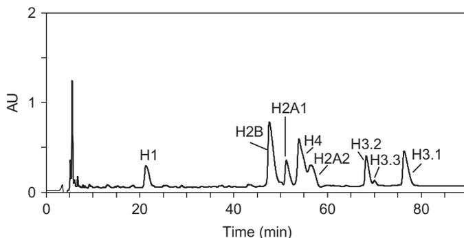
**Figure 4** Chromatogram for histone variant purification. This chromatogram was obtained by injected 200  $\mu\text{g}$  of acid-extracted histone from HeLa cells on a 4.6 mm  $\text{C}_{18}$  column. Note that other cell types may contain varying abundances of histone variants, but the elution times should remain the same. The identity of each peak is provided.
